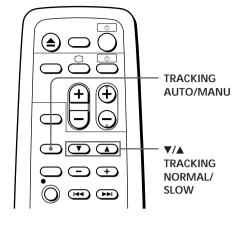
distortion should disappear as you press one of the two buttons. If you cannot get a clear picture with manual adjustment, press TRACKING AUTO/MANU to return to automatic adjustment.
