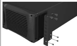
(Figure 3-a) UPS Bracket Ear Installation
