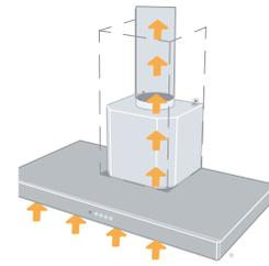
**The recycling hood filters the fumes and steam from the air and then returns it to the kitchen.**
