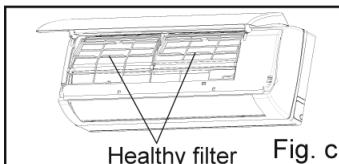
3. Mount the air filter properly along the arrow direction in Fig. d, and then close the panel cover.
