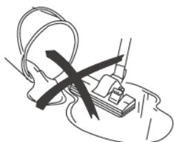
**Do not use the appliance to vacuum needles, drawing-pins, strings and sharp objects.**
