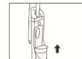
11) Twist the Quick Release Cord Wrap clockwise to unwrap the Power Cord completely and plug into a grounded outlet.
