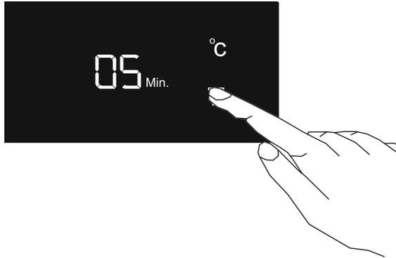
Drink cool button should be pressed to activate beverage cooling mode. Each press will increment the time for 5 minutes up to 30 minutes, and then it returns to zero. You can view the time zone you want to set on “Drink cool alarm counter” section. Drink cool mode only lets the refrigerator release an audible alert after a specific period.
