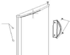
a. Remove the right bush on the upper door trim, install it to left symmetrical position.
