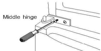
8. Place the fridge door back on. Ensure the fridge door is aligned horizontally and vertically so that the seals are closed on all sides before finally tightening the top hinge.
