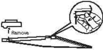
2. a. Undo the screws, lift the hinge bracket up and take it off.
