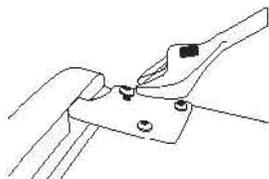
9. Put the top cover back and tighten it with the screws. Reverse step 1a to 1c for details.
