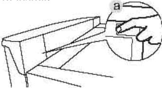
b. Take of the middle hinge by removing the screws. Lift the freezer door up and move it away.
