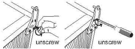
6. Remove the screw from the bottom hinge and refit it to the opposite side. Place the freezer door back on.
