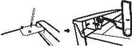
b. Remove the bolt with a screwdriver and flip the hinge bracket then reattach the bolt to the hinge bracket. Remove the fridge door.
