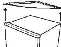
c. Remove the left hinge cover. Insert the right hinge cover.
