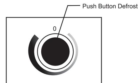
3. This refrigerator is equipped with a «push Button» (semi-automatic) defrost thermostat system. To activate the defrost cycle, simply push (in) the red defrost button located in the center of the control knob/dial. (do not turn the control knob/dial to zero=off). The defrost cycle is initiated immediately. When defrosting is complete, the «push Button» will release (pop-out) automatically and resume normal operating conditions at the same temperature setting.
