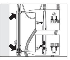
The machine must not be moved without the transit bars in place. Store them as shown or keep them in a safe place for future use. They must be re-fitted if the machine is to be moved again (e.g. when moving house).
