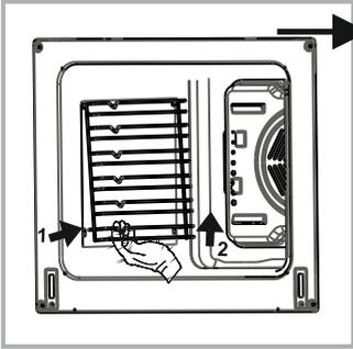
Pull the wire shelf as shown in the picture. After releasing it from clips, lift it up.
