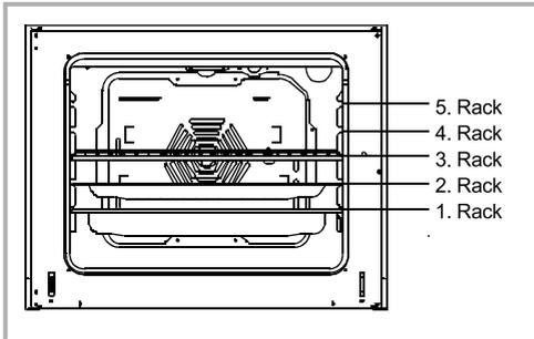
**WARNING-** Fit the grid correctly into any correspondent rack in the oven cavity and push it to the end.
