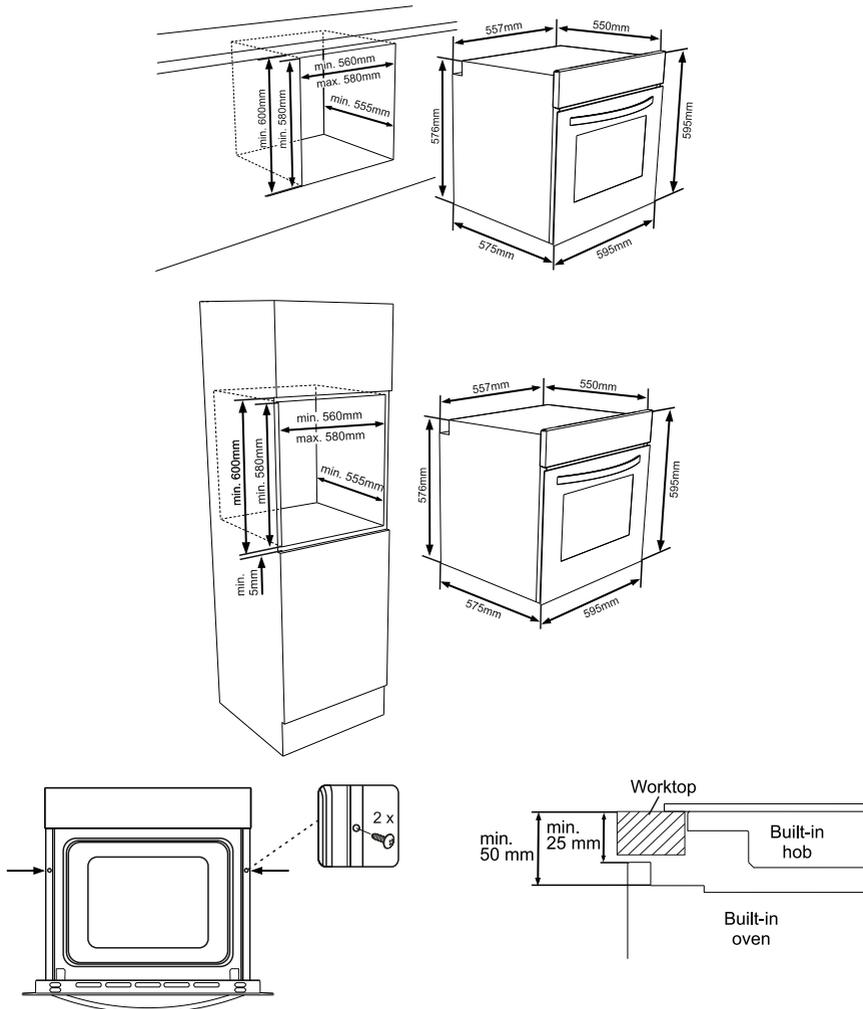
Insert the oven into the cabinet by pushing it forward. Open the oven door and insert 2 screws in the holes located on the oven frame. While the product frame touches the wooden surface of cabinet, tighten the screws.
