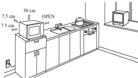
A minimum clearance of 7.5cm is required between the oven and any adjacent walls. One side must be open.
