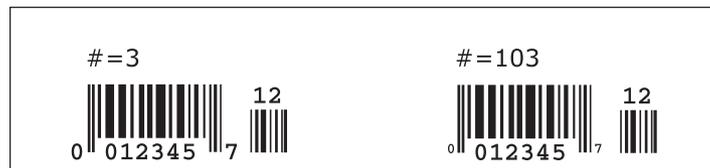
For Interleaved 2of5 +CHK, Code39 +CHK, Code128, EAN/UCC-128 and CODAR +CHKmod16, if 100 is added (# = 100@105), the check digit is printed as a human readable character.
