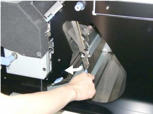
Figure 4-72. Clearing Paper from the Paper Feed Area (18)
