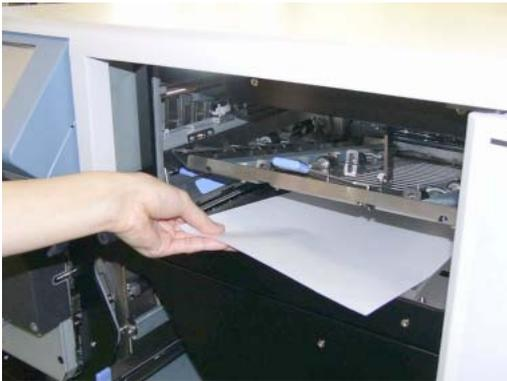
Figure 4-81. Clearing Paper from the Paper Feed Area (27)
