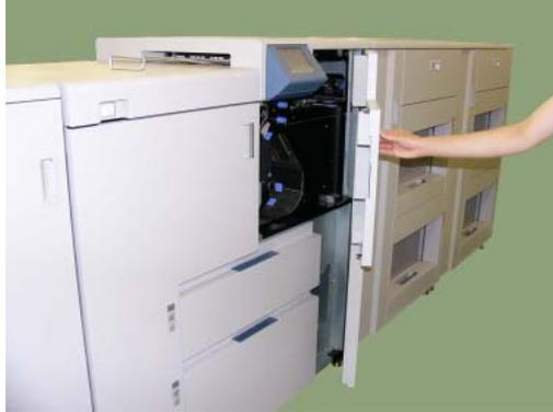
**Figure 4-116. Cleaning the Inverter Valve Piece (1)**
