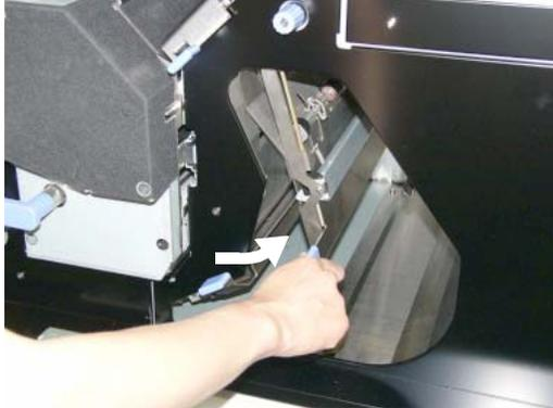
Figure 4-70. Clearing Paper from the Paper Feed Area (16)
