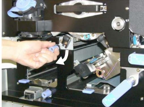
Figure 4-58. Clearing Paper from the Paper Feed Area (4)
