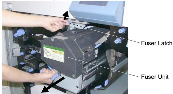
Figure 4-28. Replacing the Fuser Cleaning Web (2)
