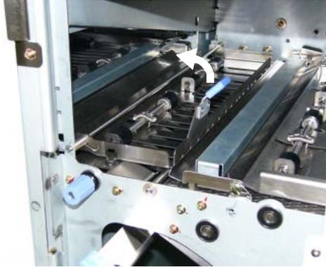
**Figure 4-86. Clearing Paper from the Container Stacker (4)**
