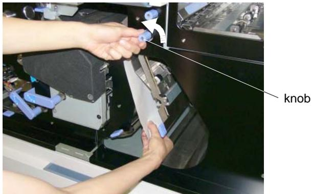
Figure 4-71. Clearing Paper from the Paper Feed Area (17)
