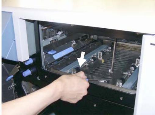
**Figure 4-82. Clearing Paper from the Paper Feed Area (28)**
