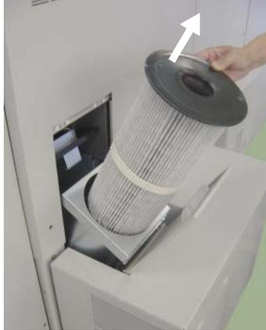
**Figure 4-36. Replacing the Fine Filter (3)**
