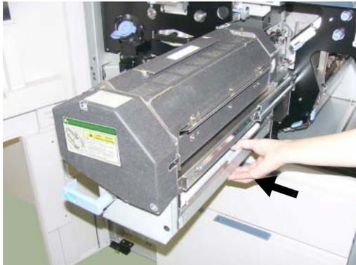
**Figure 4-31. Replacing the Fuser Cleaning Web (5)**
