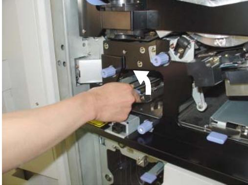
**Figure 4-76. Clearing Paper from the Paper Feed Area (22)**
