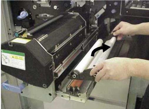
**Figure 4-30. Replacing the Fuser Cleaning Web (4)**
