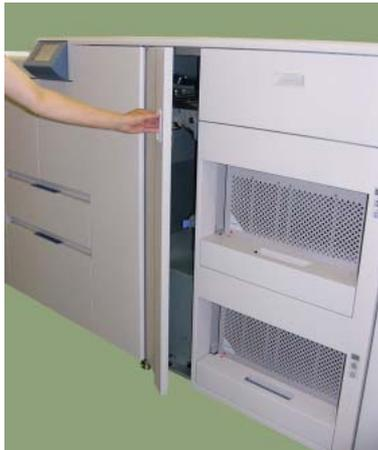
**Figure 4-84. Clearing Paper from the Container Stacker (2)**
