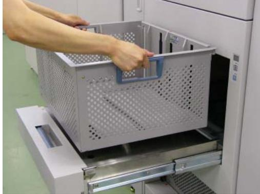
**Figure 4-92. Clearing Paper from the Container Stacker (10)**
