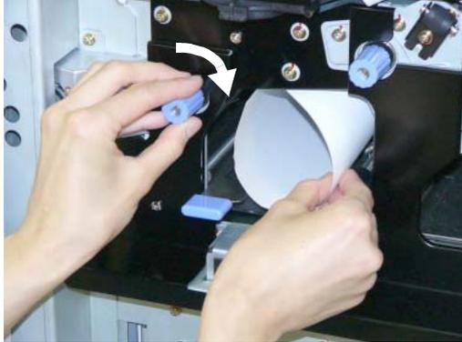
**Figure 4-54. Clearing Paper from the Regist Station Area (4)**
