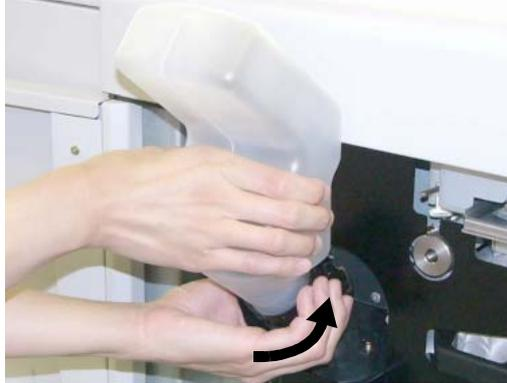
**Figure 4-26. Replacing the Developer Mix (16)**
