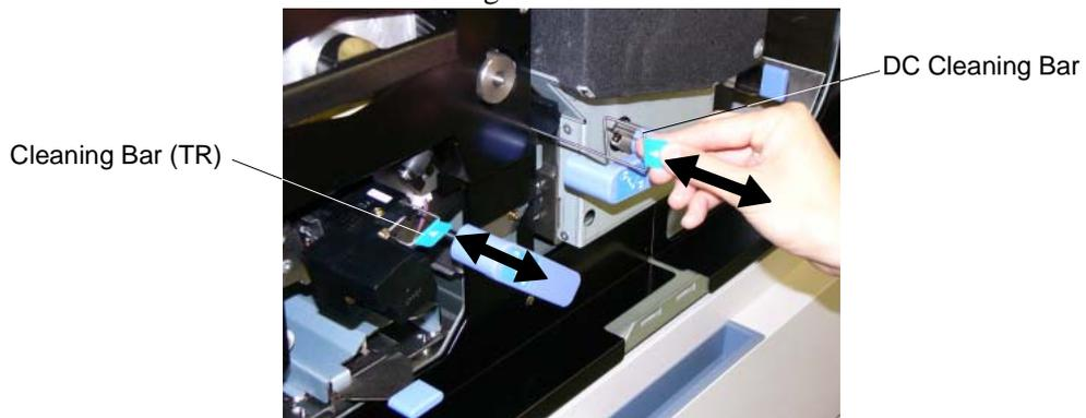
**Figure 4-115. Cleaning the Discharger and the Detach Corotron (2)**
