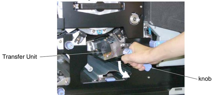
**Figure 4-57. Clearing Paper from the Paper Feed Area (3)**
