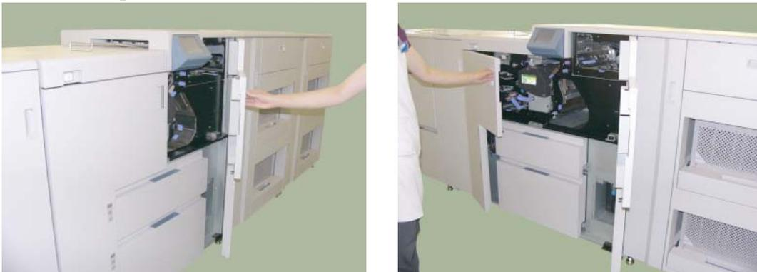
**Figure 4-56. Clearing Paper from the Paper Feed Area (2)**
