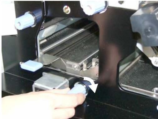
**Figure 4-74. Clearing Paper from the Paper Feed Area (20)**
