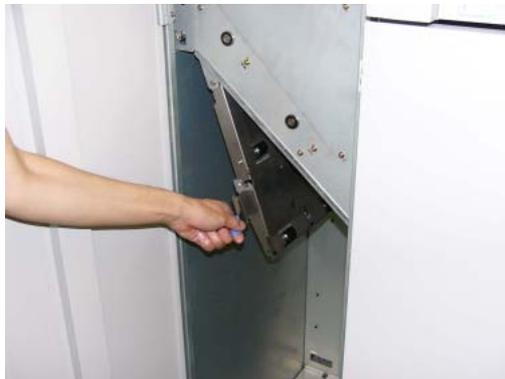
**Figure 4-100. Clearing Paper from the High Capacity Feeder (3)**
