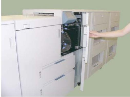
**Figure 4-8. Replacing the Toner Bag (1)**
