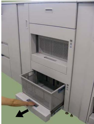
**Figure 4-93. Clearing Paper from the Container Stacker (11)**
