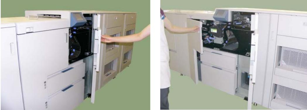
**Figure 4-114. Cleaning the Discharger and the Detach Corotron (1)**
