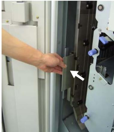
**Figure 4-102. Clearing Paper from the High Capacity Feeder (5)**
