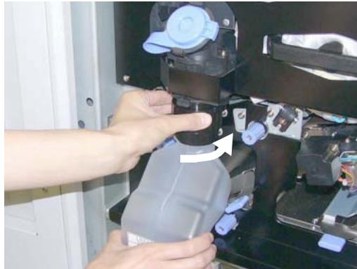
**Figure 4-13. Replacing the Developer Mix (3)**
