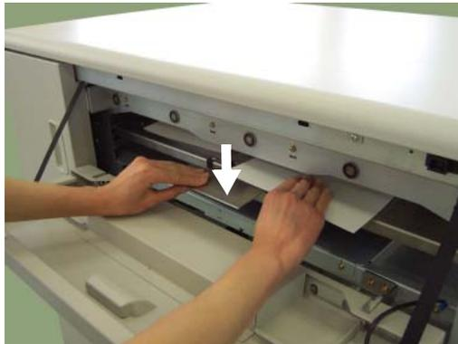
**Figure 4-105. Clearing Paper from the High Capacity Feeder (8)**
