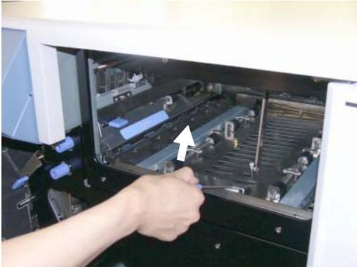
Figure 4-80. Clearing Paper from the Paper Feed Area (26)
