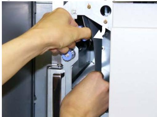
**Figure 4-103. Clearing Paper from the High Capacity Feeder (6)**
