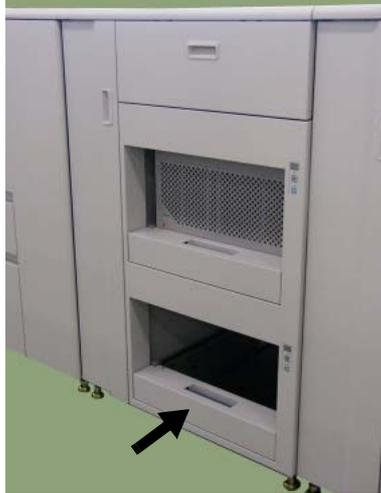
**Figure 4-94. Clearing Paper from the Container Stacker (12)**
