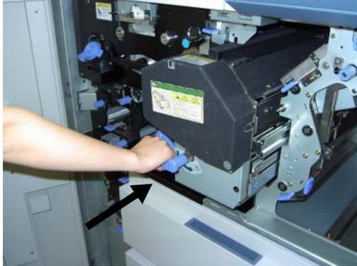
**Figure 4-32. Replacing the Fuser Cleaning Web (6)**
