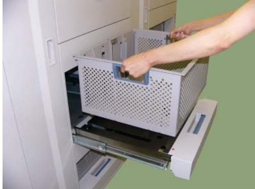
**Figure 4-111. Cleaning the Container Baskets (1)**
