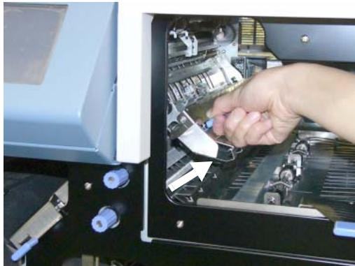
**Figure 4-77. Clearing Paper from the Paper Feed Area (23)**
