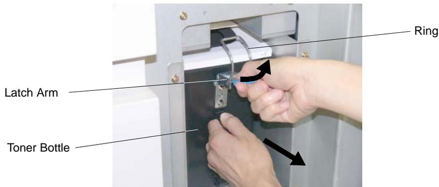
**Figure 4-9. Replacing the Toner Bag (2)**
