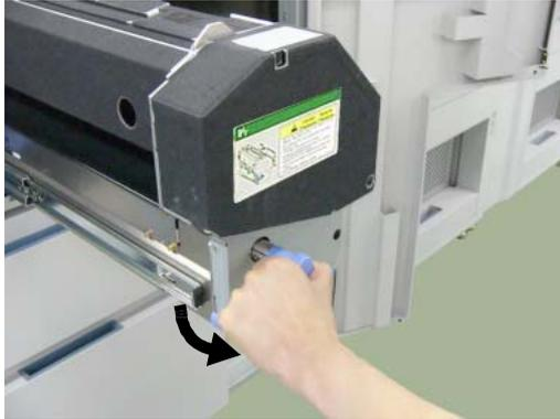
Figure 4-63. Clearing Paper from the Paper Feed Area (9)
