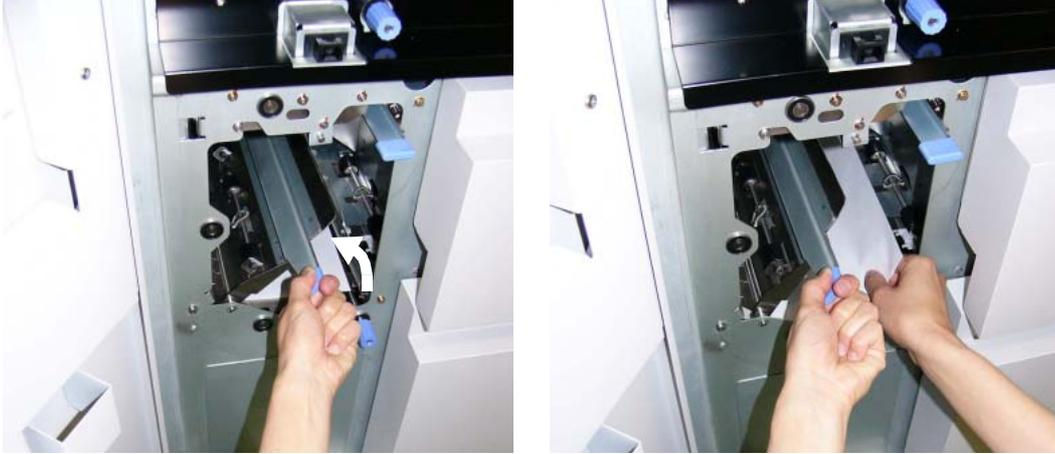
**Figure 4-49. Clearing Paper from the Input Station Area (4)**
