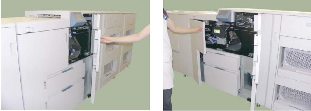
Figure 4-27. Replacing the Fuser Cleaning Web (1)
