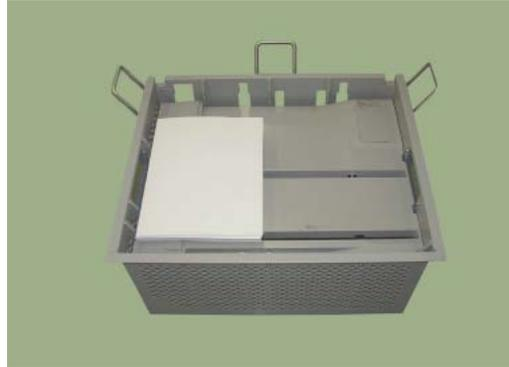
**Figure 3-41. Removing paper from the Stacker (5)**
