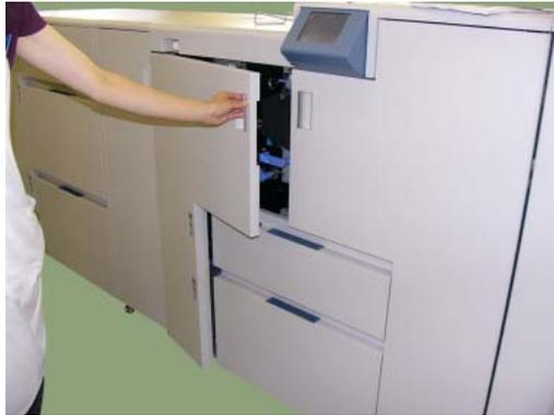
**Figure 4-47. Clearing Paper from the Input Station Area (2)**
