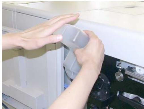
Figure 4-24. Replacing the Developer Mix (14)
