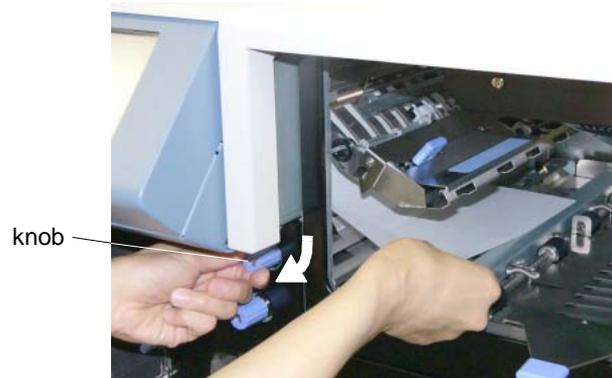
**Figure 4-78. Clearing Paper from the Paper Feed Area (24)**
