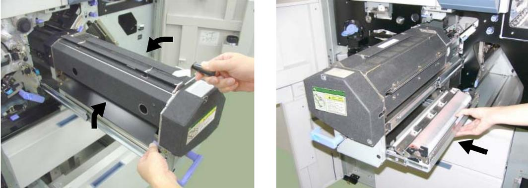
Figure 4-67. Clearing Paper from the Paper Feed Area (13)
