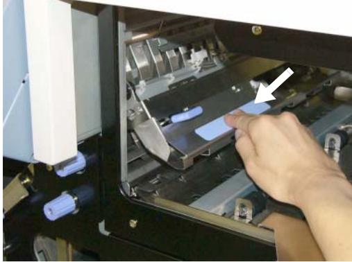
Figure 4-79. Clearing Paper from the Paper Feed Area (25)
