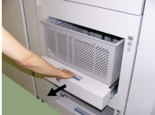
**Figure 4-89. Clearing Paper from the Container Stacker (7)**
