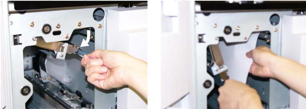
**Figure 4-50. Clearing Paper from the Input Station Area (5)**
