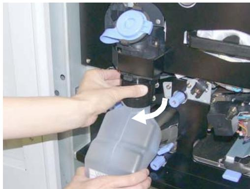
**Figure 4-17. Replacing the Developer Mix (7)**
