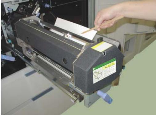
**Figure 4-66. Clearing Paper from the Paper Feed Area (12)**
