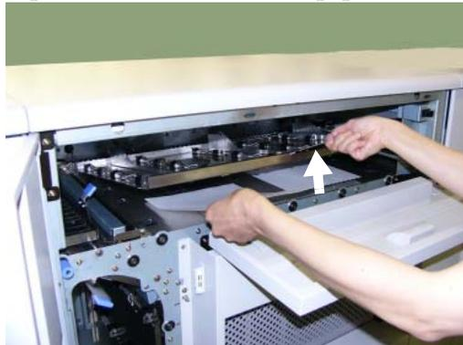
**Figure 4-97. Clearing Paper from the Container Stacker (15)**
