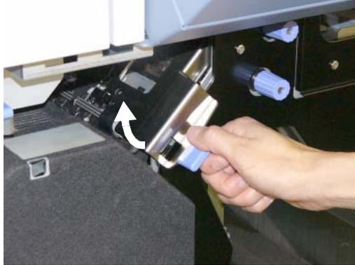
**Figure 4-61. Clearing Paper from the Paper Feed Area (7)**
