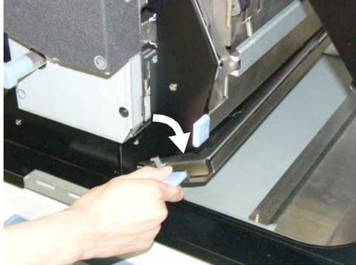
**Figure 4-73. Clearing Paper from the Paper Feed Area (19)**
