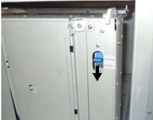
**Figure 3-12. Setting the Non-Standard Paper Size(1)**
