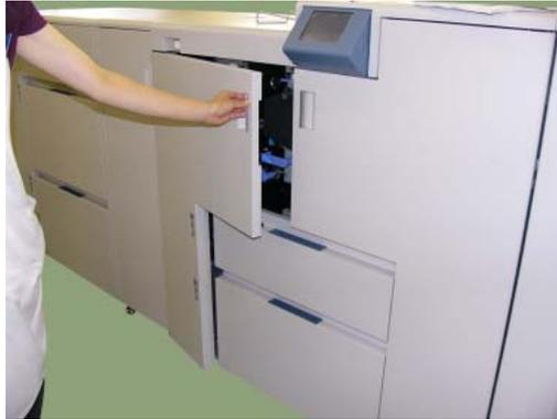
**Figure 4-52. Clearing Paper from the Regist Station Area (2)**
