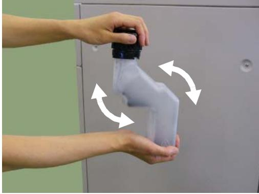
**Figure 4-18. Replacing the Developer Mix (8)**
