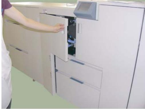
**Figure 4-11. Replacing the Developer Mix (1)**
