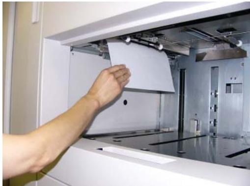
**Figure 4-91. Clearing Paper from the Container Stacker (9)**
