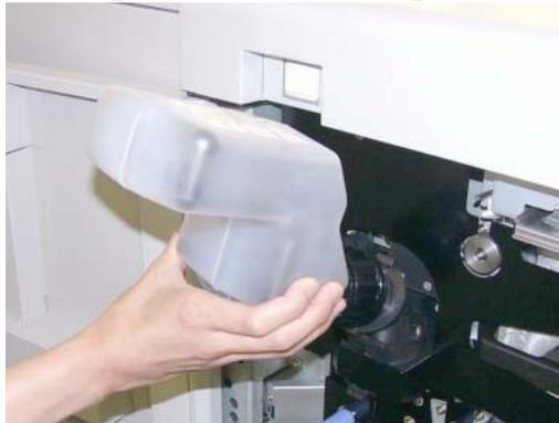
**Figure 4-20. Replacing the Developer Mix (10)**
