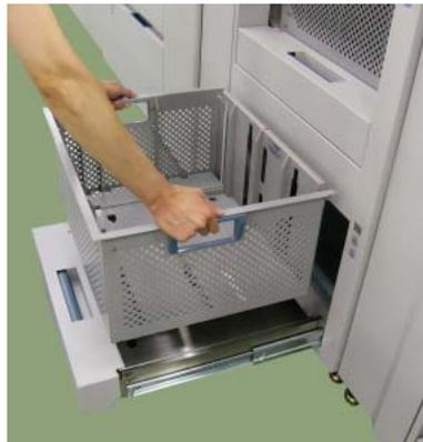
**Figure 4-95. Clearing Paper from the Container Stacker (13)**
