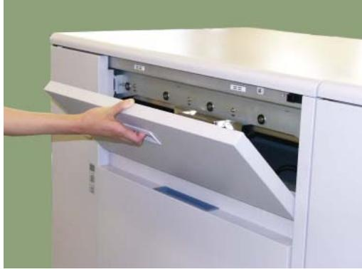
**Figure 4-104. Clearing Paper from the High Capacity Feeder (7)**
