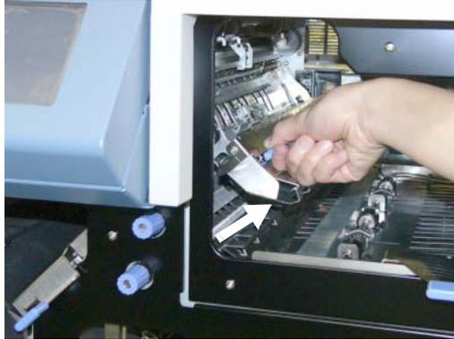
**Figure 4-117. Cleaning the Inverter Valve Piece (2)**
