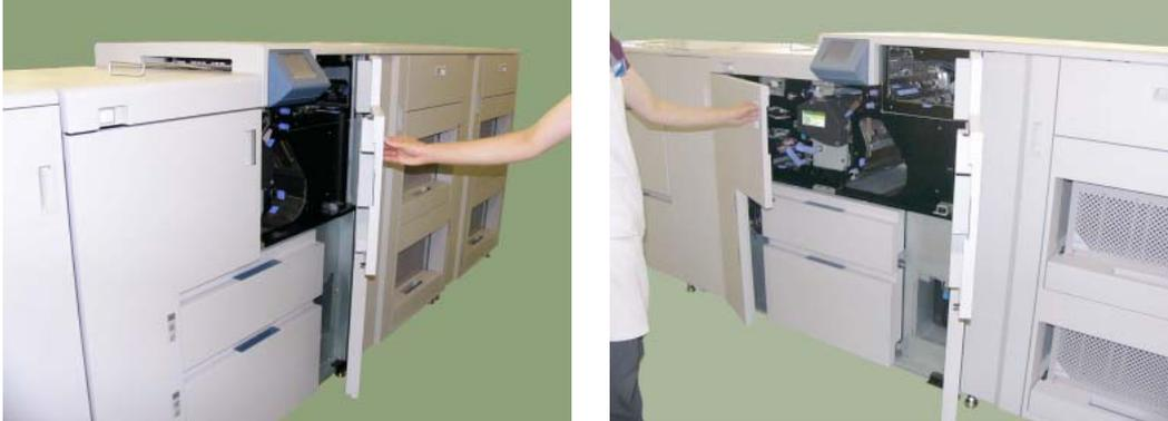
**Figure 4-120. Cleaning the paper guide of the Fuser Unit (1)**
