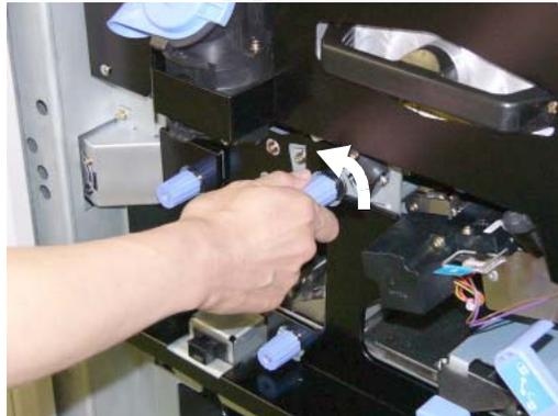
**Figure 4-53. Clearing Paper from the Regist Station Area (3)**
