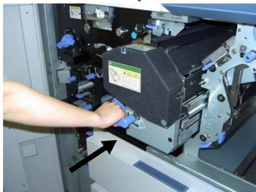
Figure 4-69. Clearing Paper from the Paper Feed Area (15)
