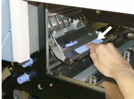
**Figure 4-119. Cleaning the Inverter Valve Piece (4)**
