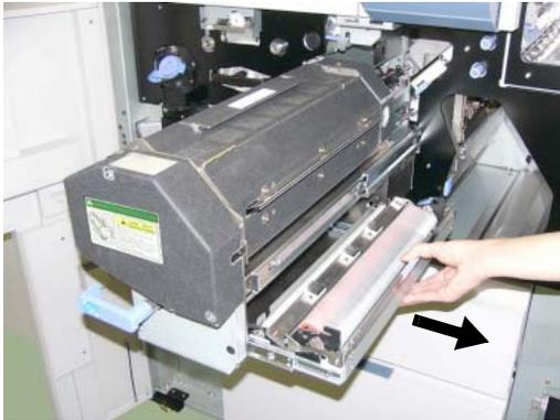
Figure 4-64. Clearing Paper from the Paper Feed Area (10)
