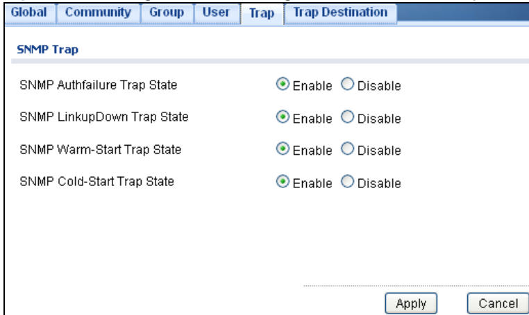
Figure 196 Configuration > Management > SNMP > Trap
