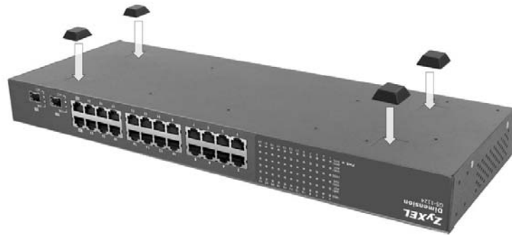
Figure 2-1 Attaching Rubber Feet
