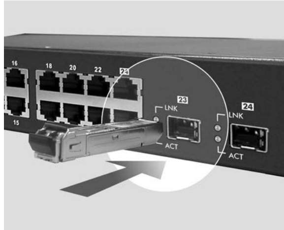
Figure 2-7 Transceiver Installation Example
