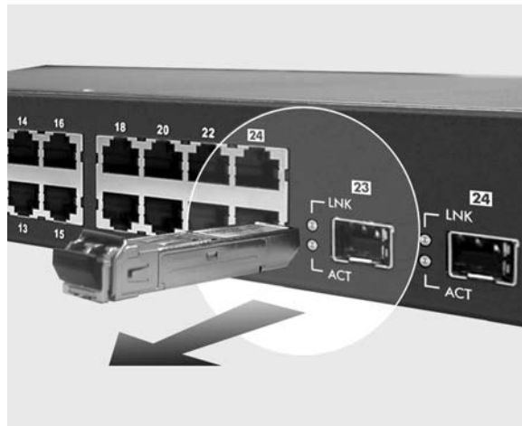
Figure 2-10 Transceiver Removal Example
