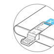
You can see the edge of the SIM card under the device cover
