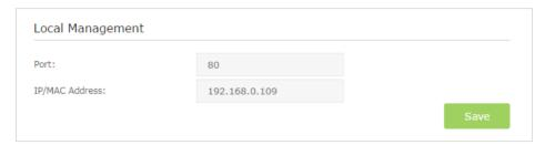
4. Click Save to make the settings effective. Now only the device using the IP address or MAC address you set can manage the router.
