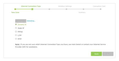
5. In this case, the router automatically detects Dynamic IP as the connection type. Click Next.
