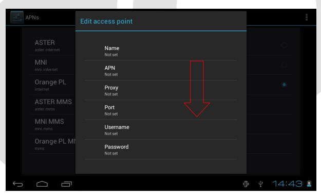
8) If parameters **MMC** and **MNC** are available tablet works with the modem correctly, now input your network provider's settings: **Name**, **APN** and **Username** also **Password** if needed. Tap to save your settings.
