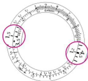
*Example 2:* if a vehicle covers 4.5 km (or 4.5 miles) in 1 minute 30 seconds (= 90 seconds), what is its average speed?
