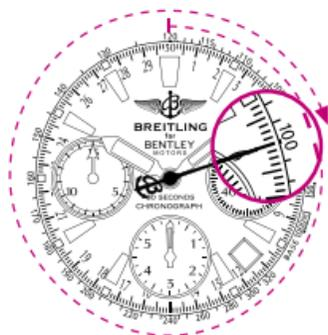
N.B. This tachometric scale, used in conjunction with the 30-seconds chronograph function, is especially suited to measuring high speeds ranging between 95 km/h (or mph) and 320 km/h (or mph). Consequently, the observation time is limited to between 11 and 38 seconds.
