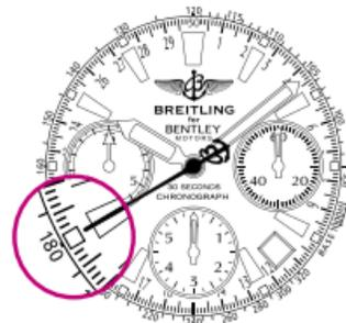
*Example 2:* if it takes 36 seconds to cover one kilometer or one mile, the average speed is 100 km/h or 100 mph respectively.
