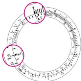
**Division:** division works in the opposite way to the previous example. To divide 54 by 2, one need only place the figure 54 opposite the HOURS mark on the fixed scale or figure 1 on the mobile disc. The result is read off opposite figure 2 on one or other of the scales. This single operation produces a complete division table of the figure 54:
