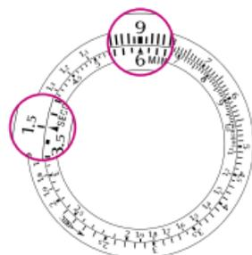
**Hourly production or consumption rate:** measuring a production rate or an hourly consumption rate follows the same principle as the measurement of an average speed. For example, if a machine produces 15 units in 45 seconds, what is its hourly production?
