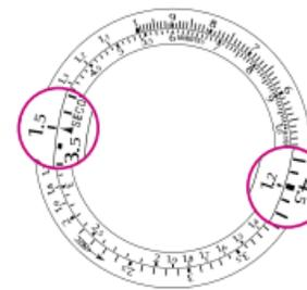
**Pulsometer:** the pulsometer enables fast calculation of pulse rate. For example, if 27 beats are measured over a 24-second period, one need only place the figure 27 (number of heartbeats) opposite the MINUTES marker, and then read off the result opposite figure 24 (length of observation); in this case 67 beats per minute.
