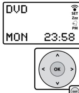
The LCD display always shows the active mode of the remote control (TV, DVD, etc.) and the current time. These indications will be displayed as long as the batteries are not worn down.
