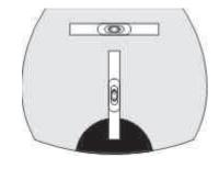
With the aid of a spirit level, screw each foot in and out until the subwoofer is
