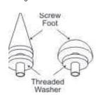
Screw the threaded washer over each foot as shown. Screw a foot part-way into the threaded hole at the bottom of each leg of the subwoofer and handtighten the washer. When all four screw feet have been fitted, stand the subwoofer upright and remove the bag.
