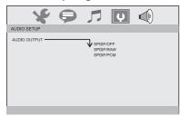
The function is used to select the SPDIF output: SPDIF Off, SPDIF/RAW. SPDIF/PCM.
