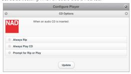
**Always Rip:** Loaded audio disc will be directly ripped to the connected M52 or USB mass storage device.
