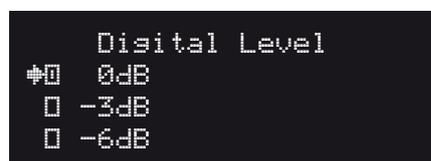
Select "Digital Level" to attenuate output level by -3dB or -6dB. The default level is 0dB.
