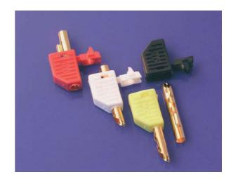
Our **banana plugs** are manufactured using a special byrillium copper sheet and subsequently gold plated. The byrillium gives the copper the necessary spring tension that is needed in order to ensure a high contact pressure when in contact with a socket and therefore guaranteeing security. The acoustic advantages of copper remain largely unaffected.
