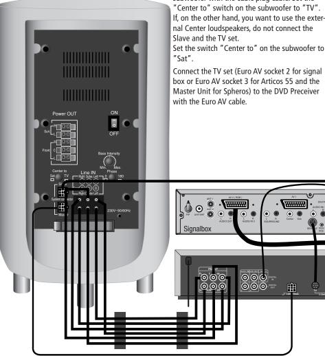
Connect the cubic socket on the DVD Preceiver to the "Master" cubic socket on the Tremo subwoofer. Use the cubic plug cable provided with the DVD Preceiver Auro (2-wire cable). Plug the white plug (without kink protection) into the cubic socket on the subwoofer.
