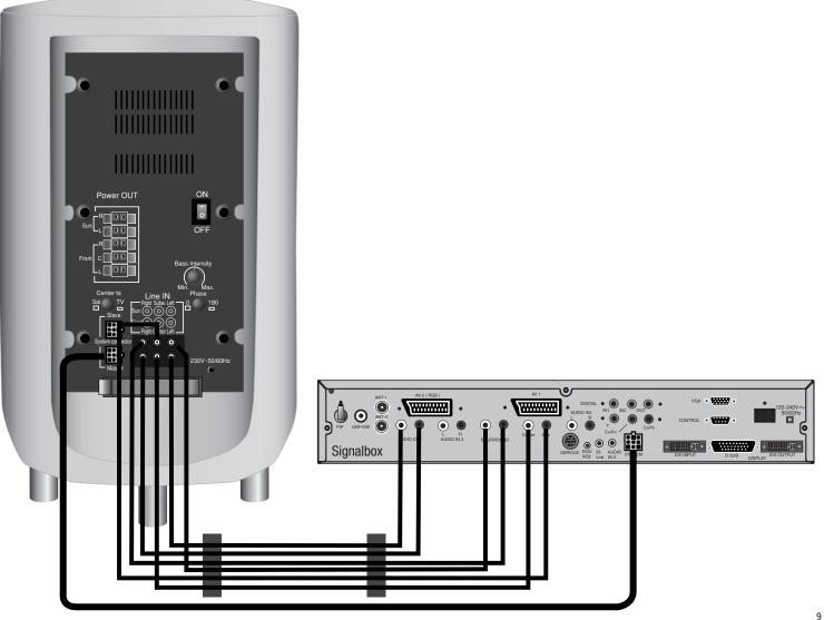
... to Loewe DVD Preceiver Auro 8116 DT with Loewe TV set (from Loewe TV MediaPlus Q2500, software 6.x) If you use the Loewe DVD Preceiver in connection with a Loewe TV set, connect the Tremo speaker system to the audio outputs of the DVD Preceiver. See the instructions for laying the cables on page 6.
