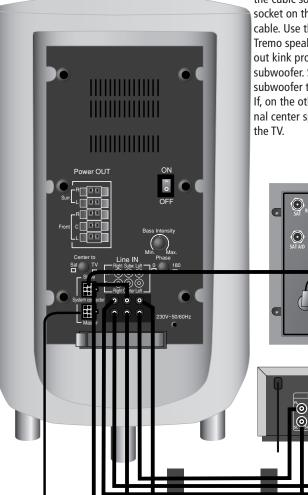
Connect the cubic socket on the DVD Preceiver to the "Master" cubic socket on the Tremo subwoofer. Use the cubic plug cable provided with the DVD Preceiver Auro (2-wire cable). Plug the white plug (without kink protection) into the cubic socket on the subwoofer.
