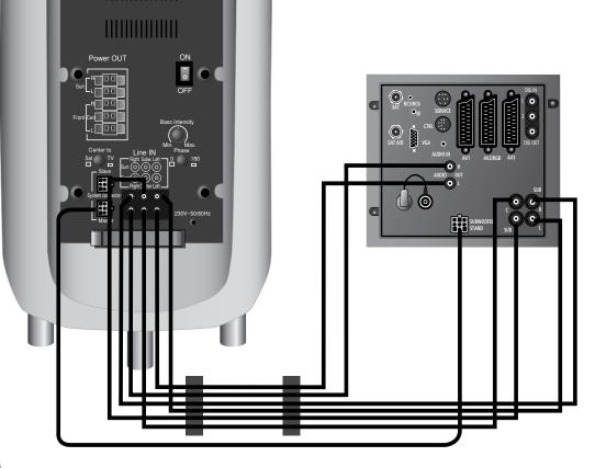
... to Articos 55 with Dolby Digital Module (from software version 6.20) See the instructions for laying the cables on page 6. The "Center" connections do not necessarily have to be made because the center signal is always played over the TV speakers.
