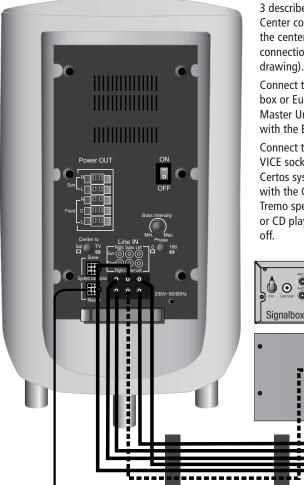
With the connecting cable order no. 88947.001 connect the bass module link socket to the Certos system with the cubic socket "Master" on the Tremo subwoofer.
