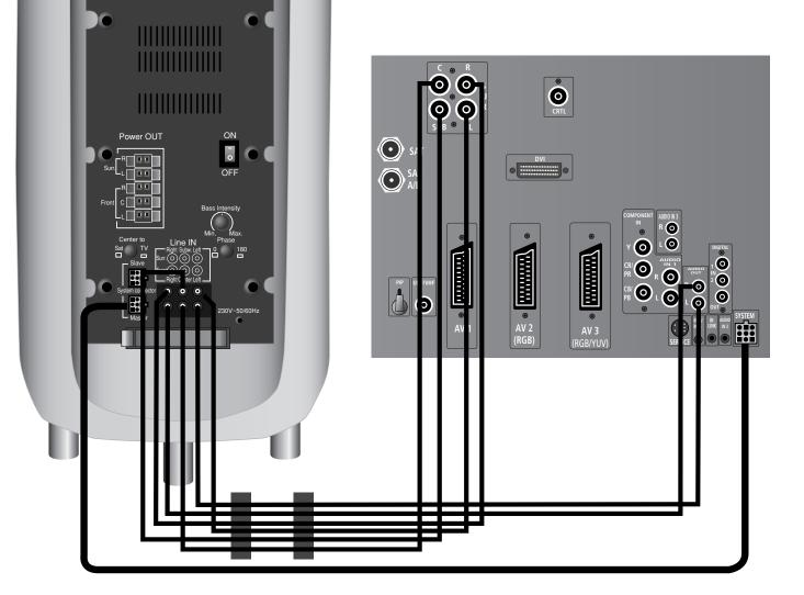
... to the Master Unit with Dolby Digital Module with Spheros 42 HD and Spheros 37 (from software version 6.14) See the instructions for laying the cables on page
