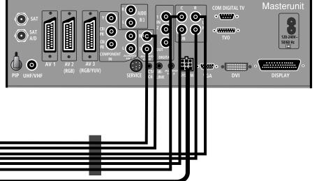
... to TV sets with the signal box with builtin Dolby Digital Module
