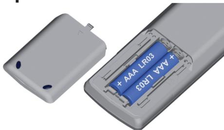
To insert or change the batteries, press on the arrow. While doing so, simply slide the battery compartment lid down and remove it. Insert alkali manganese batteries LR 03 (AAA) and ensure the correct position of + and -. Slide the cover on again from the bottom.
