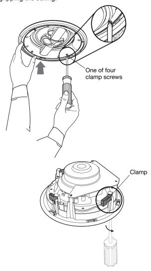
**CAUTION:** Tighten these screws firmly, but avoid using so much pressure that the clamps compress the ceiling material. This can cause the material to crumble, creating an uneven surface with gaps between the speaker face and the ceiling.
