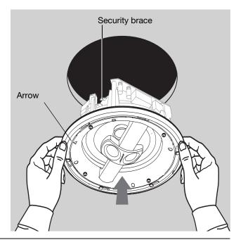
**CAUTION:** Be careful not to damage or remove any of the foam gasket material along the edge of the speaker. This gasket is important to the operation of the speaker.
