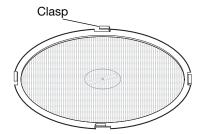
**3.** On the rim of the speaker, notice the six slots that the clasps fit into.
