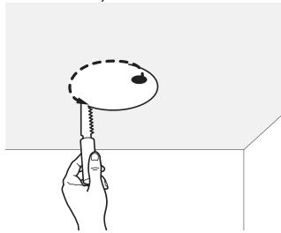
**3.** Place one hand under the circle to brace it and complete cutting the hole.
