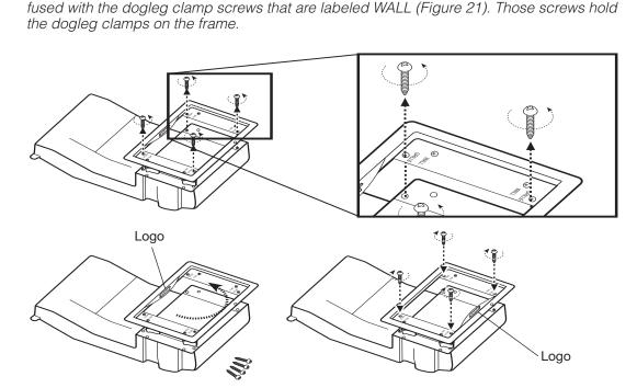
**I** Note: To position the logo right-side-up if you insert the speaker upside-down, remove the outer frame from the face of the speaker, rotate it 180°, then reattach the frame. There are four
