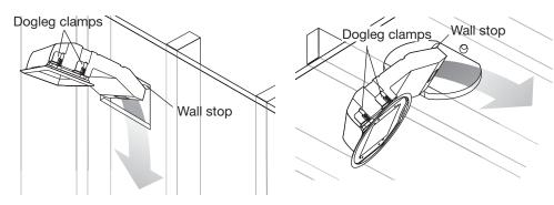
3. Leave the speaker in this partially inserted position, resting on the wall stops that prevent it from falling out (Figure 28). This allows ready access to the connection terminals on the upper left-hand side of the speaker.
