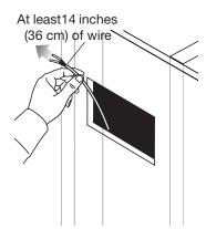
2. Use tape or the assistance of another person to temporarily affix the loose end of the wire above and to the left of the hole (Figure 26). This keeps the wire out of the way until you have the speaker partially inserted in the wall and are ready to make the connections.
