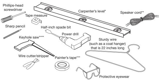
\*Carpenter's level is suggested for use when installing speakers in a wall.
