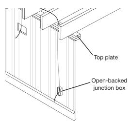
If you must route cord around a corner, you will need to cut out a rectangular piece of wallboard on either side of the joist at that corner. Use each regular-shaped cutout as the patch for the wall when you finish. By reaching through the cutout, you can notch the joist to make room for the cord and use nail plates to cover the cord in each notch (Figure 13a).
