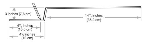
*Tip:* For greater accuracy, make the first bend a little long, measure again, and cut off the extra length at that end.
