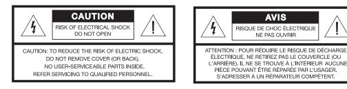
The lightning flash with arrowhead symbol within an equilateral triangle alerts the user to the presence of uninsulated dangerous voltage within the system enclosure that may be of sufficient magnitude to constitute a risk of electrical shock.
