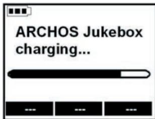
While charging, the Jukebox Recorder can be used after an hour. Charging time may then be increased up to 15 hours depending on the extent of use.
