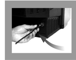
Connect the end of the coaxial cable to the TV's RF input socket.
