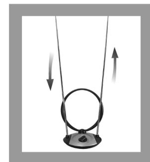
When receiving UHF signal (470-860 MHz) adjust the loop to the best reception angle.
