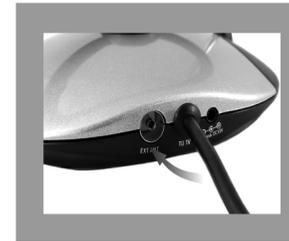
DC Connect the AC adaptor to the jack at the back of the antenna and plug the AC adapter into a standard AC outlet.
