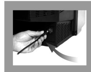
Connect the end of the coaxial cable to the TV's RF input socket.
