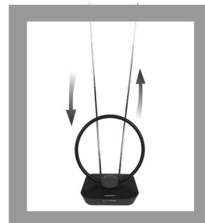
When receiving UHF signal (470-860 MHz) adjust the loop to the best reception angle. When receiving VHF signal (47-230MHz), extend and move the dipoles to the best reception.
