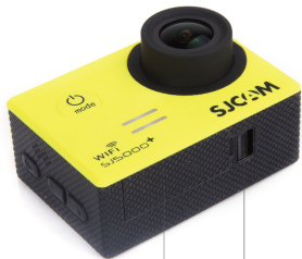
Battery door Battery door key
